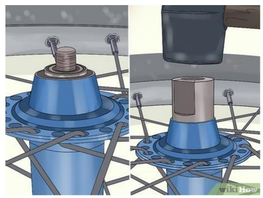
Slide the other bearing over the top side of the axle. Let the bearing sit on top of the hub opening. Then place the drift over the bearing and tap it until the bearing enters the hub.[27]
