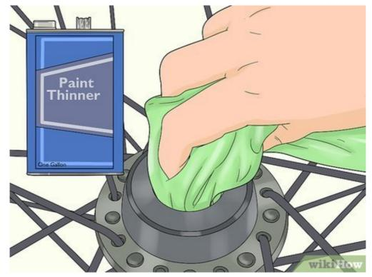
**Clean the wheel hub with paint thinner.** Pour some paint thinner onto a clean rag and wipe the inside and outside of the hub, which is the tunnel that the axle slides through. Make sure to clean out the threads on the end of the hub as well, since grease is usually trapped in there. [6]
