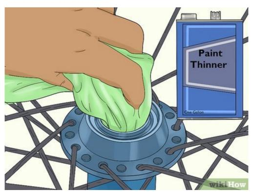
**Clean the bike hub and pieces you removed with paint thinner.** Pour some paint thinner onto a clean rag and wipe it around the hub to remove any grease buildup. Also soak the axle, caps, and other piece you removed in a jar of the solvent you use for 5 minutes to clean them. Wipe them dry afterward.[19]
