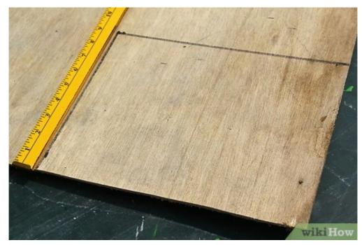
? Transfer these measurements to a piece of plywood.
