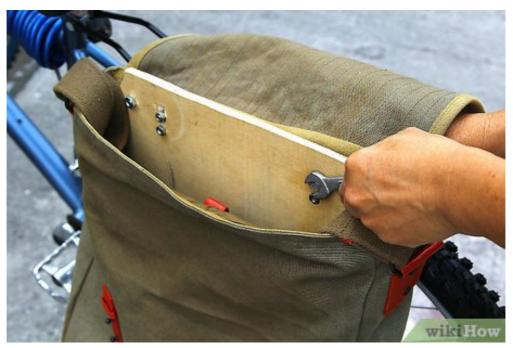
12 Secure the saddlebag to the rack by tightening the nut of the U-bolt.
