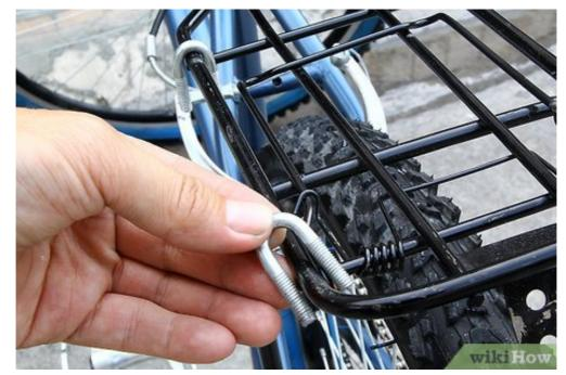
10 Prepare the rear rack. Get your U-bolt and place them on the rack. It is better you place the saddlebag on you left side of the bike so it won't interfere with any moving part of the bike, like the sprocket.
