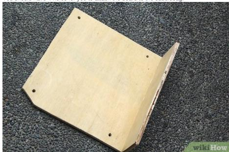
• Drill another set of holes for the U-bolts so you can mount the saddlebag to the bike rear rack.
