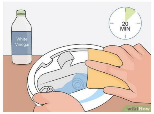
**5** Soak the base and reservoir with vinegar and water as an alternative. Empty out any remaining water in the reservoir and pour 2 tablespoons (30 mL) of white vinegar and 17 fluid ounces (0.50 L) of tap water into the reservoir. Do the same for the base. Let it sit for 20 minutes and then rinse both parts until you don't smell any signs of the vinegar.[11]
