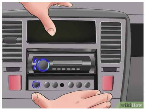
**Replace the receiver.** Put the receiver back into its bracket and place the frame covering back into place. Be sure all the wiring is pushed inside the dash beforehand.
