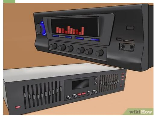
Hook up your equalizer to your receiver if it does not have preamp-out channels. The equalizer should always be between the receiver and the amplifier. Your amplifier will need integrated preamp-out and preamp-in connections to work with this method.
