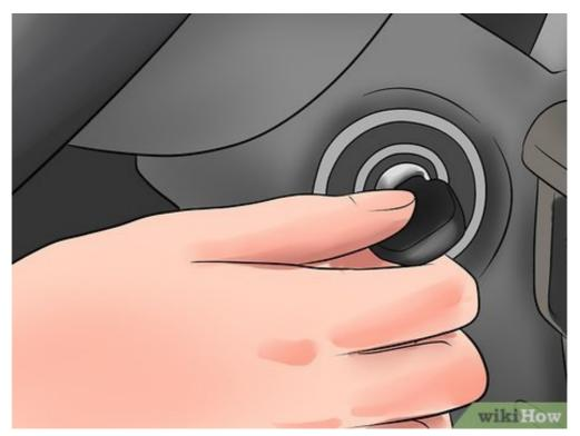
12 Test the equalizer by turning on the car. Put the key in the ignition and turn it to the "on" position. Then turn on the radio to check that everything is working well and that the equalizer turns on with the radio.
