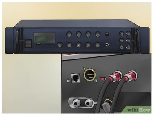
**4** Connect the other pair of RCA cables between the amplifier and receiver. Connect the other pair of cables from the output channels on the back of the equalizer to the preamp input channels on the amplifier.
