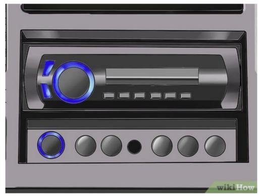
**Decide where you would like to install the equalizer.** The best place to install an indash equalizer is right above or below your head unit, or stereo control unit. Some vehicles will have space for this in their dash. Other vehicles will not have space and the equalizer can then be mounted under the dash. The final option is to custom-fit your equalizer into the dash.
