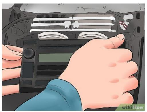
**Remove your receiver from the dash.** Remove your receiver from the dash so that you can access the wires behind. Usually you can pull off the plastic piece covering the dash and then pull the receiver slightly out.
