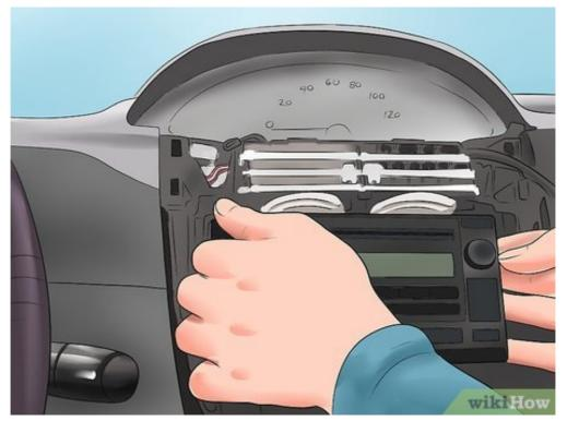
**4** Remove your receiver from the dash. Remove your receiver from the dash so that you can access the wires behind. Usually you can pull off the plastic piece covering the dash and then pull the receiver slightly out.
