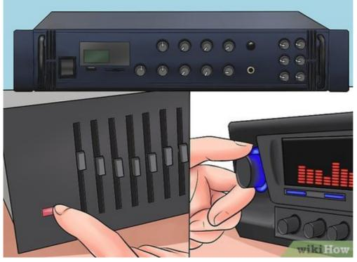
**Turn on the receiver, equalizer and amplifier to use your equalizer.** Turn on all three components and adjust the equalizer knobs according to your preferences. You should now be able to manipulate the controls on the equalizer to change the frequency response or tone of your music.
