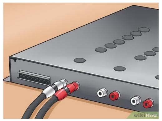
**6** Bring the cables to the equalizer and plug in. Route the cables through the dash to the equalizer. You should use tape or wire ties along the way to connect the two cables together. Plug the cables into the preamp inputs on your equalizer.[1]
