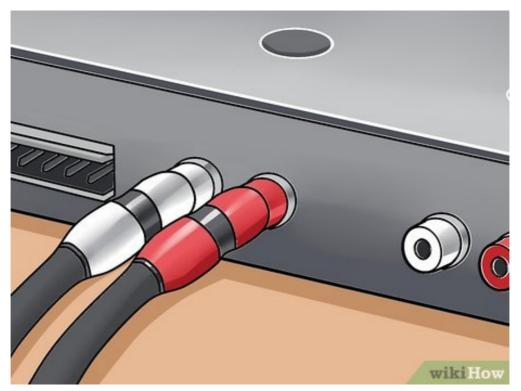
**6** Bring the cables to the equalizer and plug in. Route the cables through the dash to the equalizer. You should use tape or wire ties along the way to connect the two cables together. Plug the cables into the preamp inputs on your equalizer.
