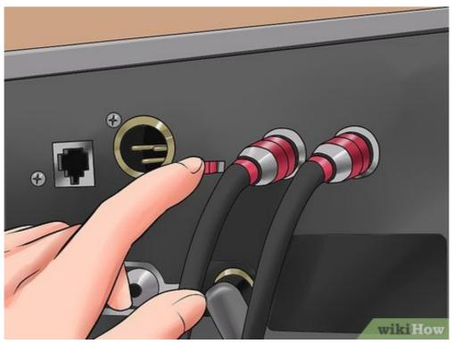
**5** Switch on the pre-amp connection on the amplifier. Some amplifiers will have a switch to turn on the pre-amp connections. If you are using tape monitor channels then you will also need to switch on the tape monitor switch. Depress the button to turn on this connection.
