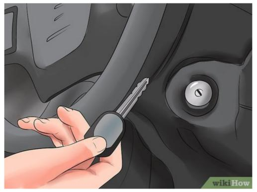
**Turn off your ignition.** Turn off your ignition completely and remove your keys before you begin installation. This is for your safety while you connect the wires to avoid getting shocked.
