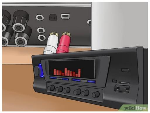
**5** Connect the amp to the receiver. The amplifier should remain connected to the receiver with an RCA cable between the amplifier outputs and the amp inputs on the receiver. This effectively creates a loop from the receiver through the equalizer and amplifier and back to the receiver.
