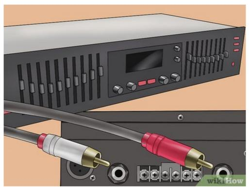
4 Connect the other pair of RCA cables between the receiver and equalizer. Connect the other pair of cables from the output channels on the back of the equalizer to the tape monitor input channels on the back of the receiver.
