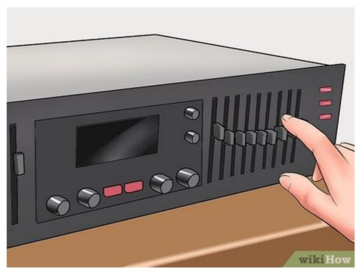
**5** Use your equalizer. Turn on the receiver and switch the front panel output control to the "Tape Monitor" setting. This opens the tape monitor channels and means that the sound will travel through your equalizer before being sent to the amplifier. Adjust the equalizer knobs according to your preferences.
