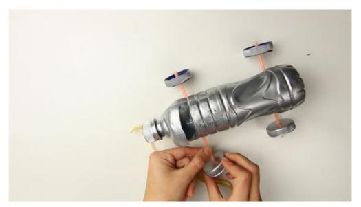
10 Place the bottle caps onto the axles of the car. Run the axles through the holes you drilled in the bottle caps. See how the car sits. If the lids are too big or too small, then the car may not move. Have the top of the lids face the car so that it has more stability.
