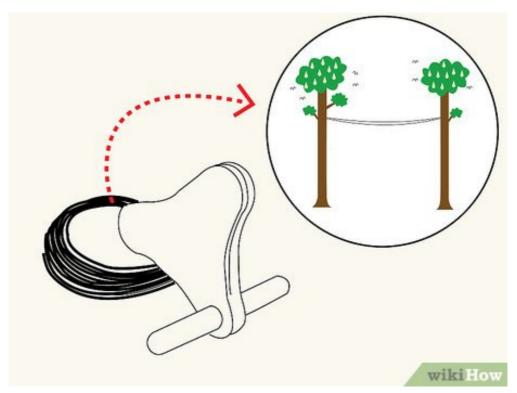
**2** Lay the cable out between the two points. You will need enough cable so there is suitable slack when it's stretched out between the two points. This slack should form a belly in the cable between the points. You **never** want to stretch the cable too tight. [2] This creates a dangerous situation of speed and crashing at the other end, and your last words will be, "Hey, watch this!" before you're taken to the hospital.
