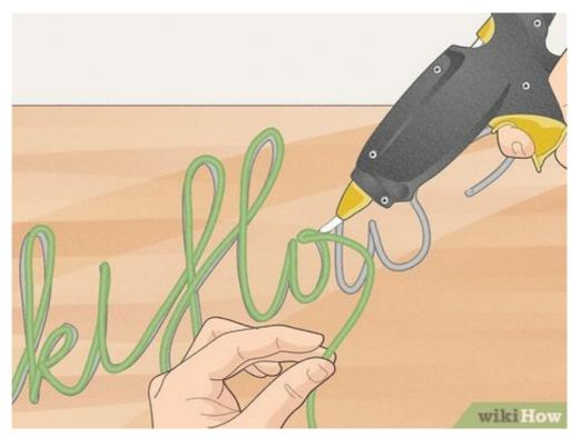
**5** Using your EL wire and a hot glue gun, glue the EL wire to the metal wire. Do this section by section. Work slowly and hold the EL wire down to the metal wire for 5-10 seconds to make sure that it is set in place.
