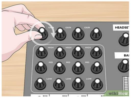
4 Use the gain knobs to continue increasing the volume of specific channels. The gain knobs are usually located at the top of each channel and are labeled "Gain." Slowly adjust the gain knob for the channel that you want to boost the audio for and test it compared to the rest of the instruments to see if you can clearly hear it.
