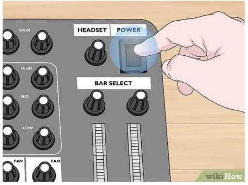
**Turn on your mixer using the power switch.** The power switch is usually on the back of the mixer or on the top right by the other knobs. Check that all of the volume and fader controls are still turned down before flipping the switch to turn it on. You will see a light turn on as soon as the power is connected. [5]
